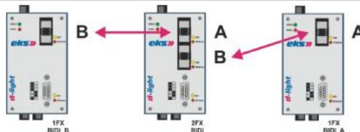
Systems with BIDI transceivers always have to be connected from transceiver type A to a transceiver type B (note the label on the back of the device). Switches with 2 FX-Ports always have transceiver type A as the upper one.
